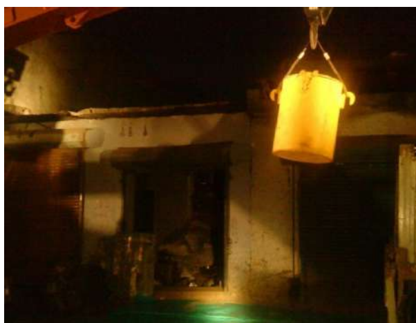
Figure 18. Shielded Flask Used for Safe Collection and Transport of Radiological Material.
