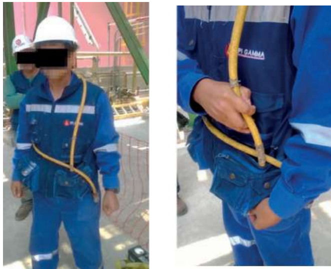
Figure 15. Placement of Guide tube and Collimator in vest pocket.
